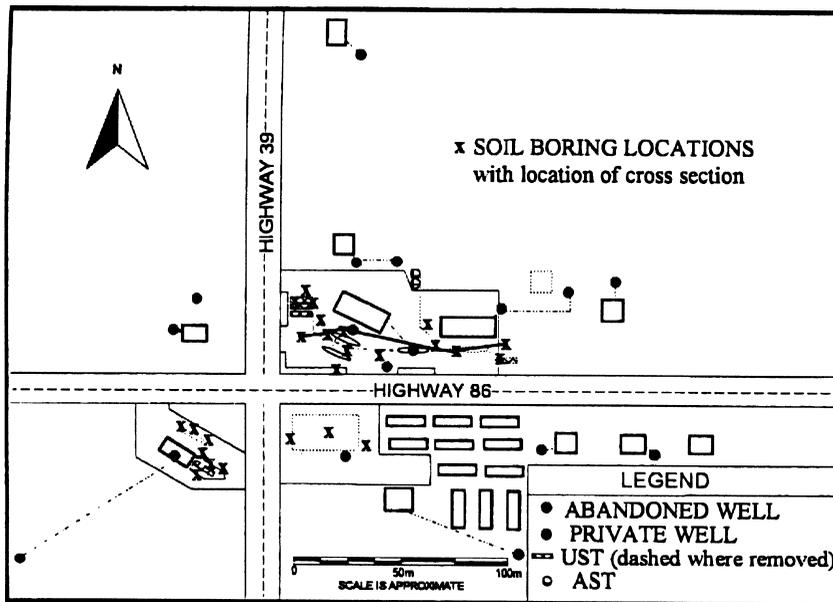
Fig. 1. Site map showing location of boreholes and the boreholes which were used to construct a cross-section.
