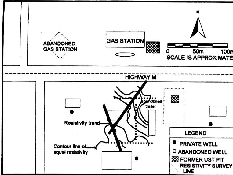
Fig. 4. Resistivity trends found in a surface resistivity geophysical survey. Subsequent drilling found the trends to be related to bedrock lows, or valleys.
