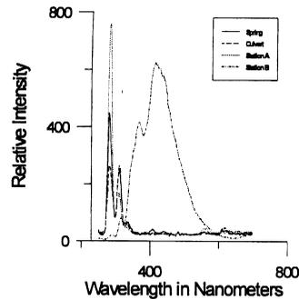
Fig. 5. Results of petroleum fingerprinting analysis performed on a synchronously scanning spectrofluorometer. The scan from contamination at Station A is similar to the scan from a contaminated spring and nearby culvert. The scan from Station B is drastically different.
