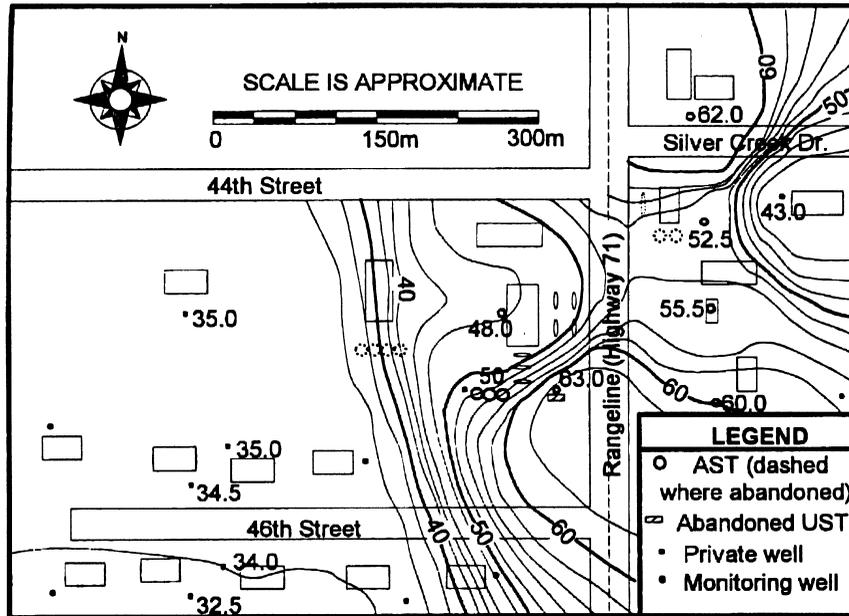
Fig. 3. Potentiometric map showing fracture induced flow. An east–northeast fracture forms a trough in the water table on both sides of the groundwater divide.
