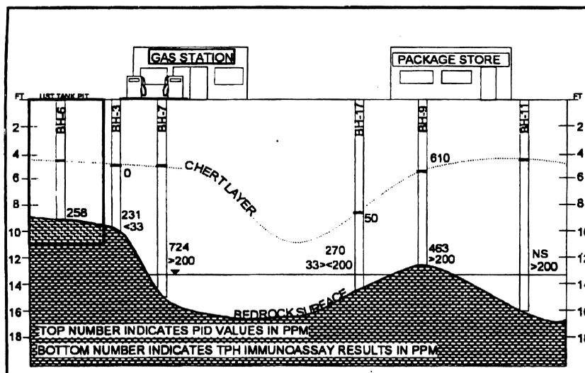
Fig. 2. Cross-section made from borehole data. Soil gas and soil sample results show contamination concentrating in bedrock lows.
