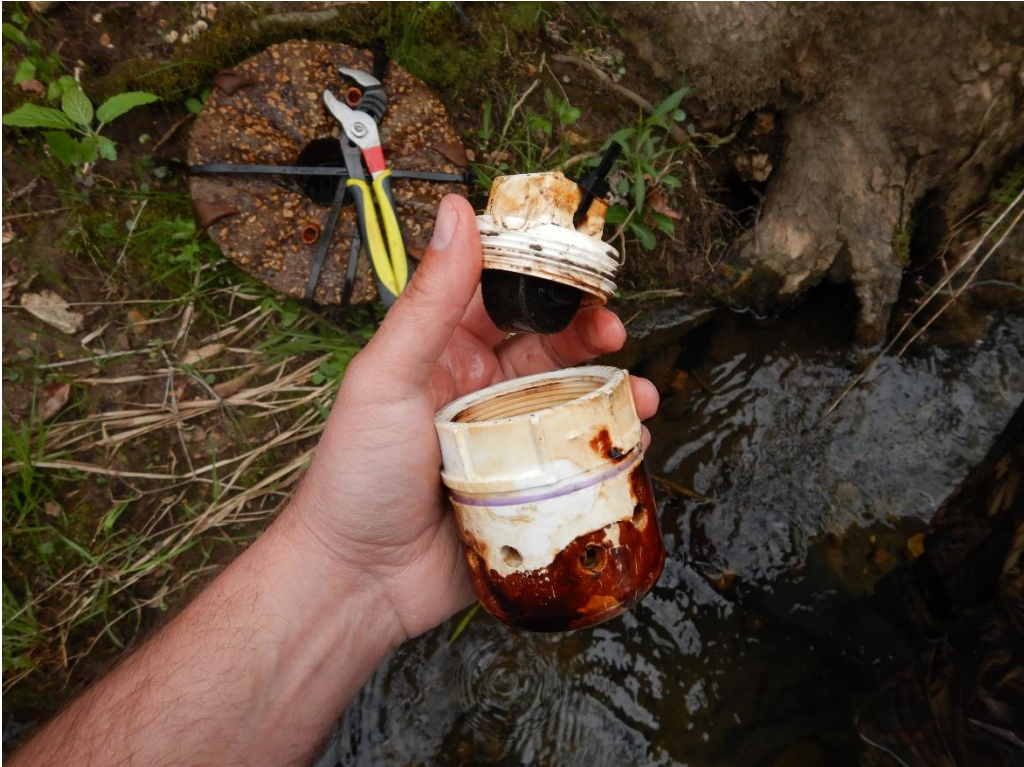
Photo 7. Temperature sensor inside secured inside PVC pipe (April 14, 2021).
