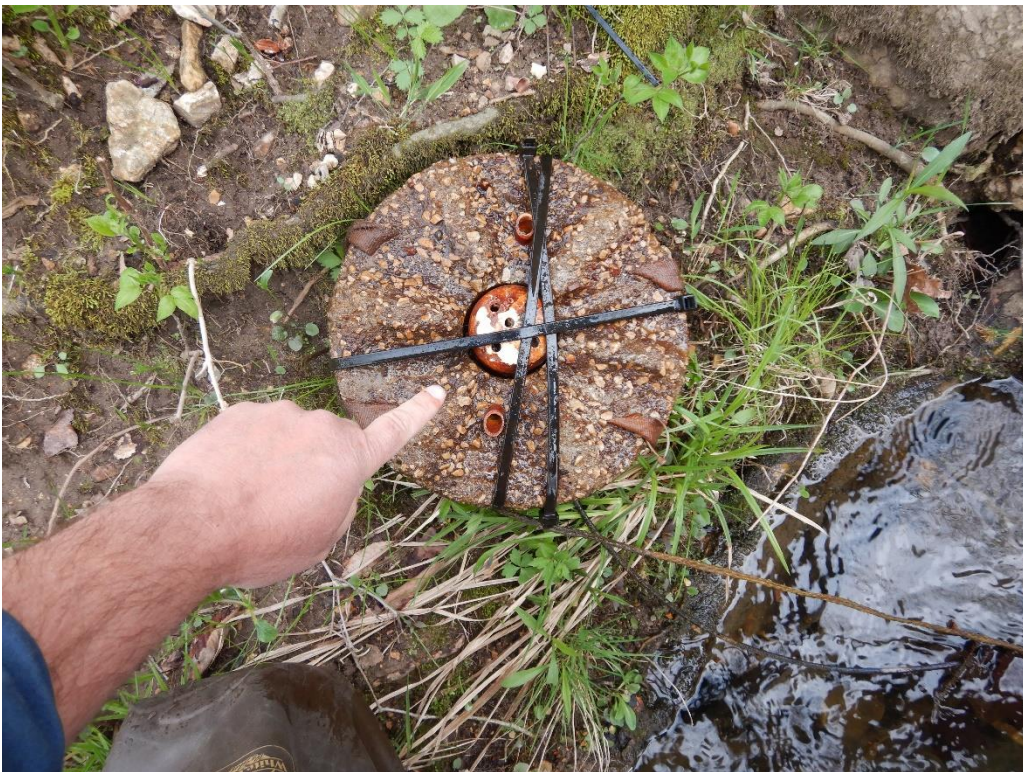
Photo 5. Temperature sensor inside PVC pipe and concrete housing (April 14, 2021).
