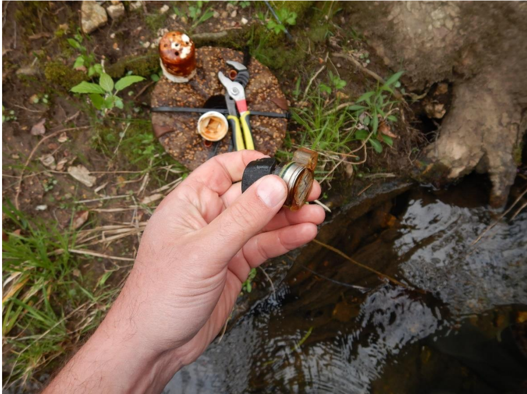
Photo 9. Temperature sensor is removed from rubber boot (April 14, 2021).
