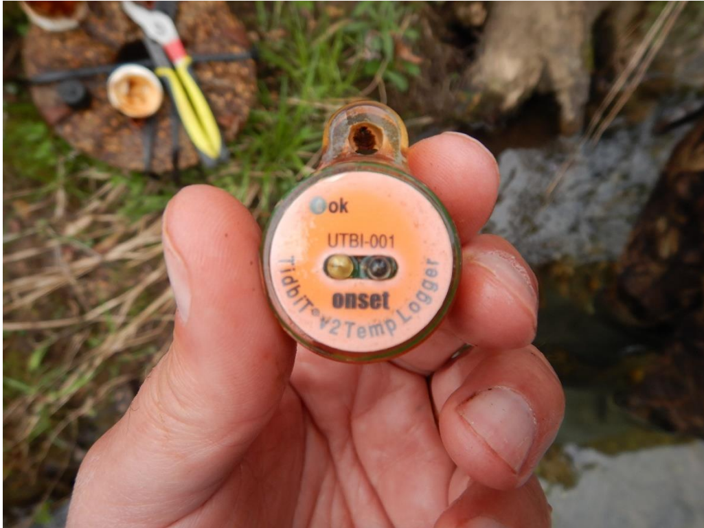
Photo 10. The Onset Hobo TidbiT Temperature Logger (April 14, 2021).
