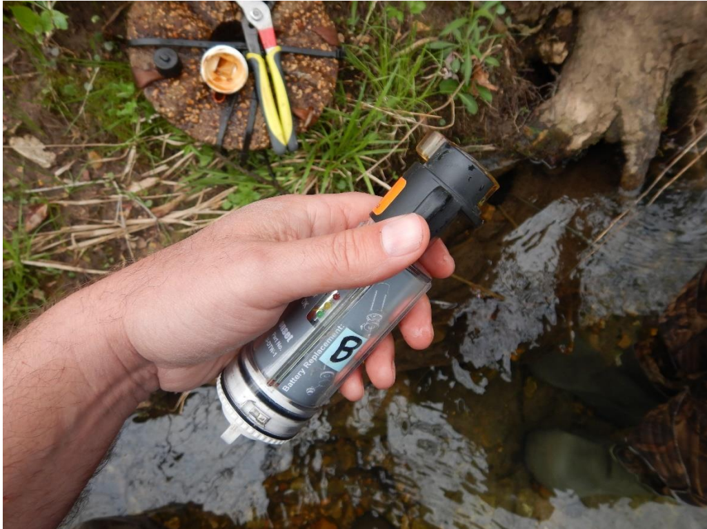
Photo 11. Temperature logger data is downloaded by waterproof shuttle (April 14, 2021).
