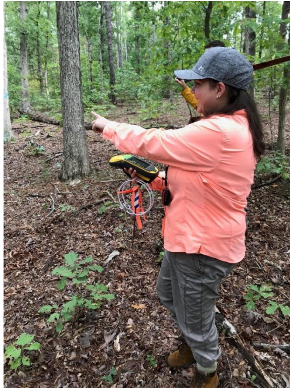
Photo 1. Using GPS navigation to locate pre-selected point locations (Swayback: Sept. 26, 2018).
