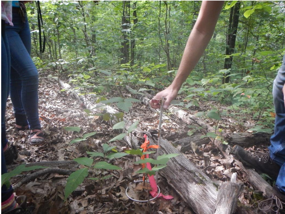
Photo 3. Measuring forest floor depth (Sterling Hollow: July 31, 2018).
