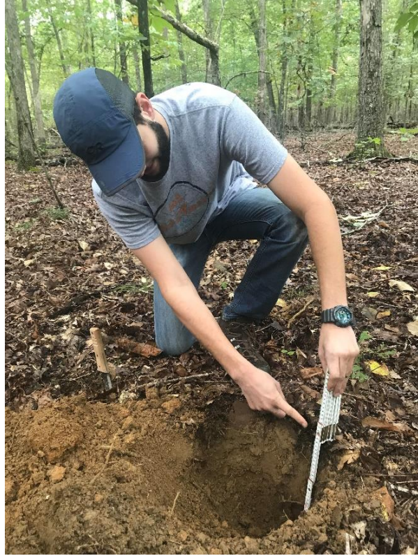
Photo 5. Measuring pit depth (Coyote: Sept. 27, 2018).
