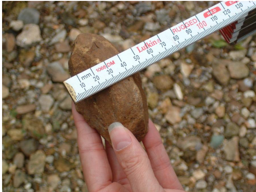
Photo 1: Measuring the B axis of a piece of sediment.
