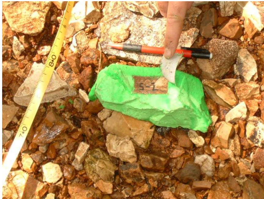
Picture 6: Showing identification number of sediment tracer
