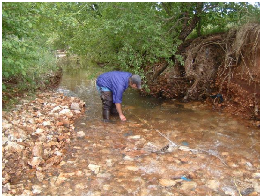
Photo 4: Recovering tracers after a storm event and measuring distance traveled
