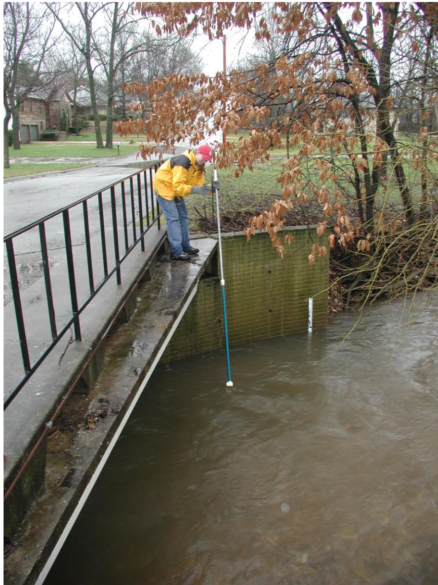
Graduate student Maya Hirsch takes velocity measurements at Camino Ave.
