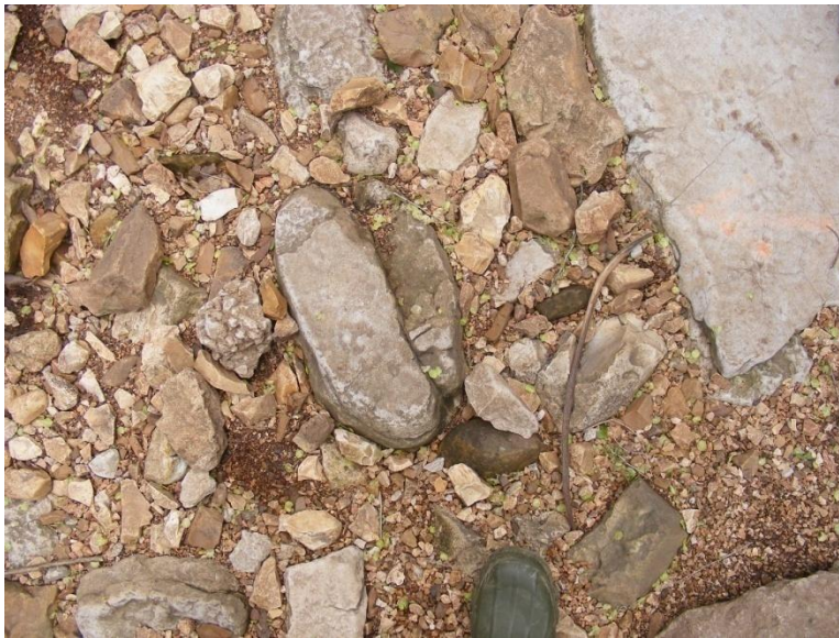
Photo 31. Fine to medium gravel fill between cobble and boulder size material near station 500 feet SR-1 (4/6/09)
