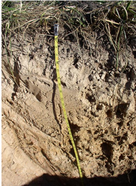
Photo 1. Soil pit #1 from the head slope landscape position showing silty texture from loess parent material over older reworked loess sitting on top of a fragipan.
