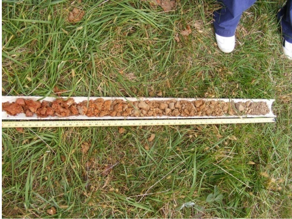
Photo 13. Example of a Soil Profile at the Project Site (Loess over Colluvium over Residuum) (October 2008)
