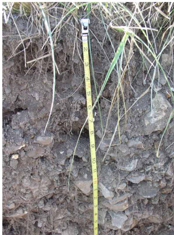
Photo 6. Soil pit from the valley bottom landscape position with unconsolidated rocky colluvial parent material that may be result of past land clearing.
