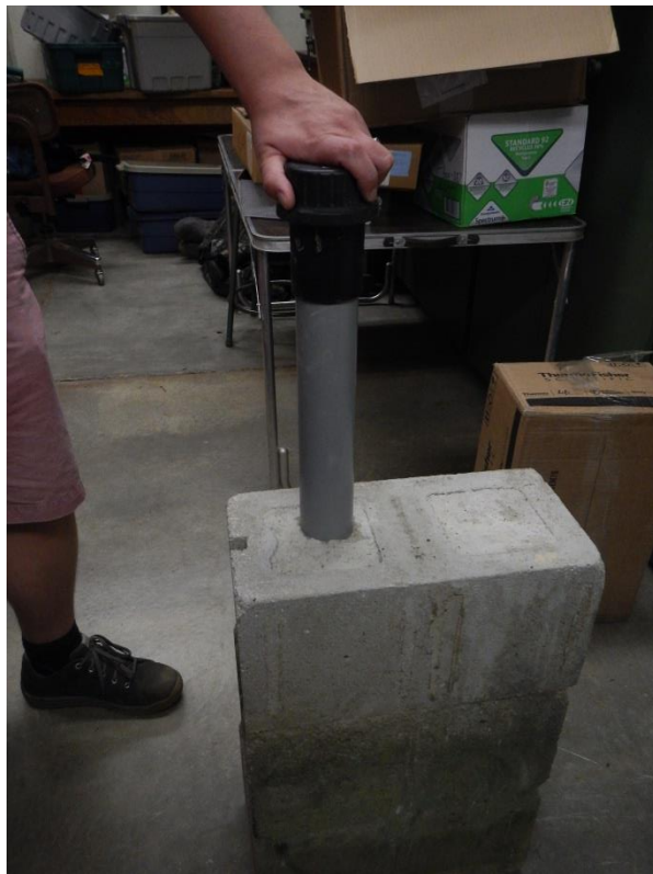
Photo 6. Levellogger housing with cap.
