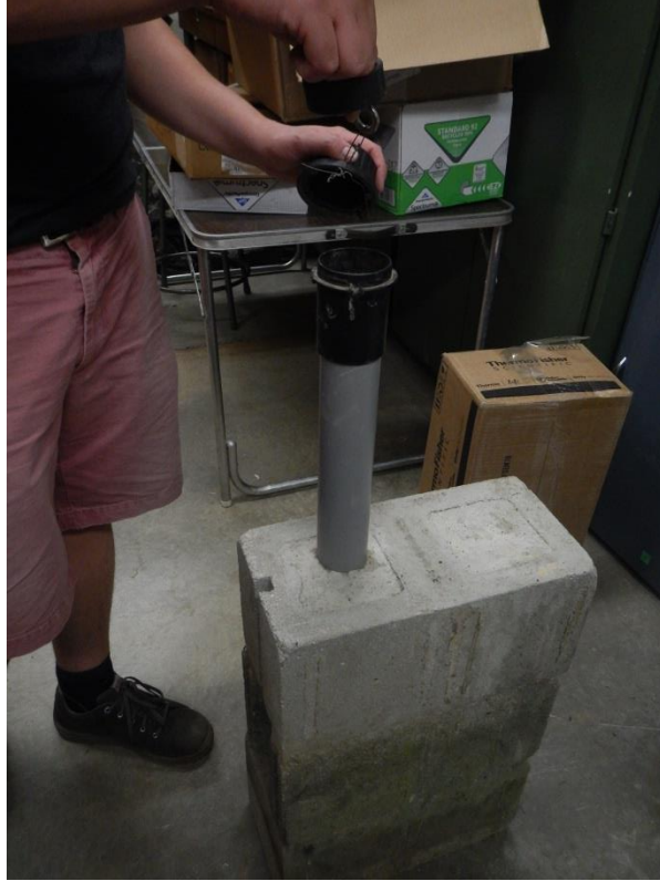
Photo 7. Removing levellogger from housing.
