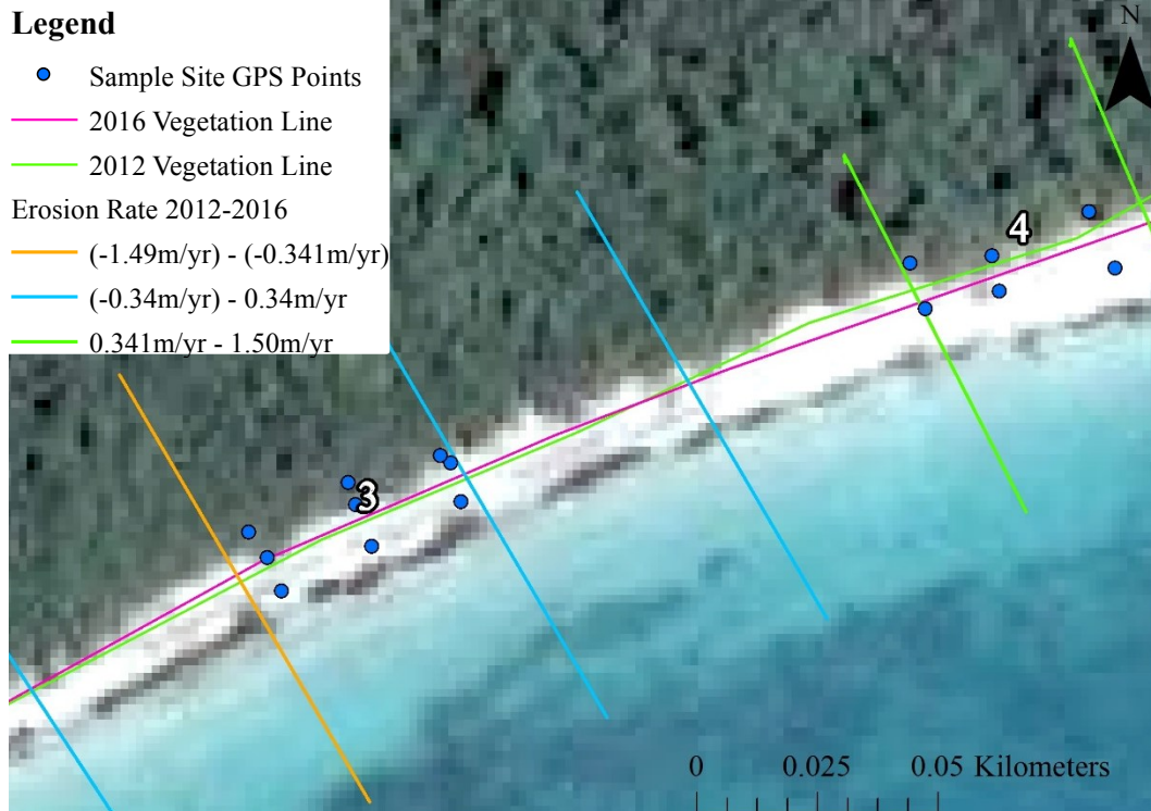
Figure 12: Method used to determine the updated erosion rates for Galleon Fish Sanctuary. The vegetation line for 2012 and 2016 was digitized and the distance between the lines was measured. The base map is from 2016 (Google Earth Pro, 2016).
