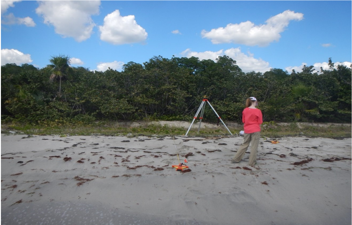
Survey set up with auto level on berm crest, tape pinned with 10 m at berm crest.
