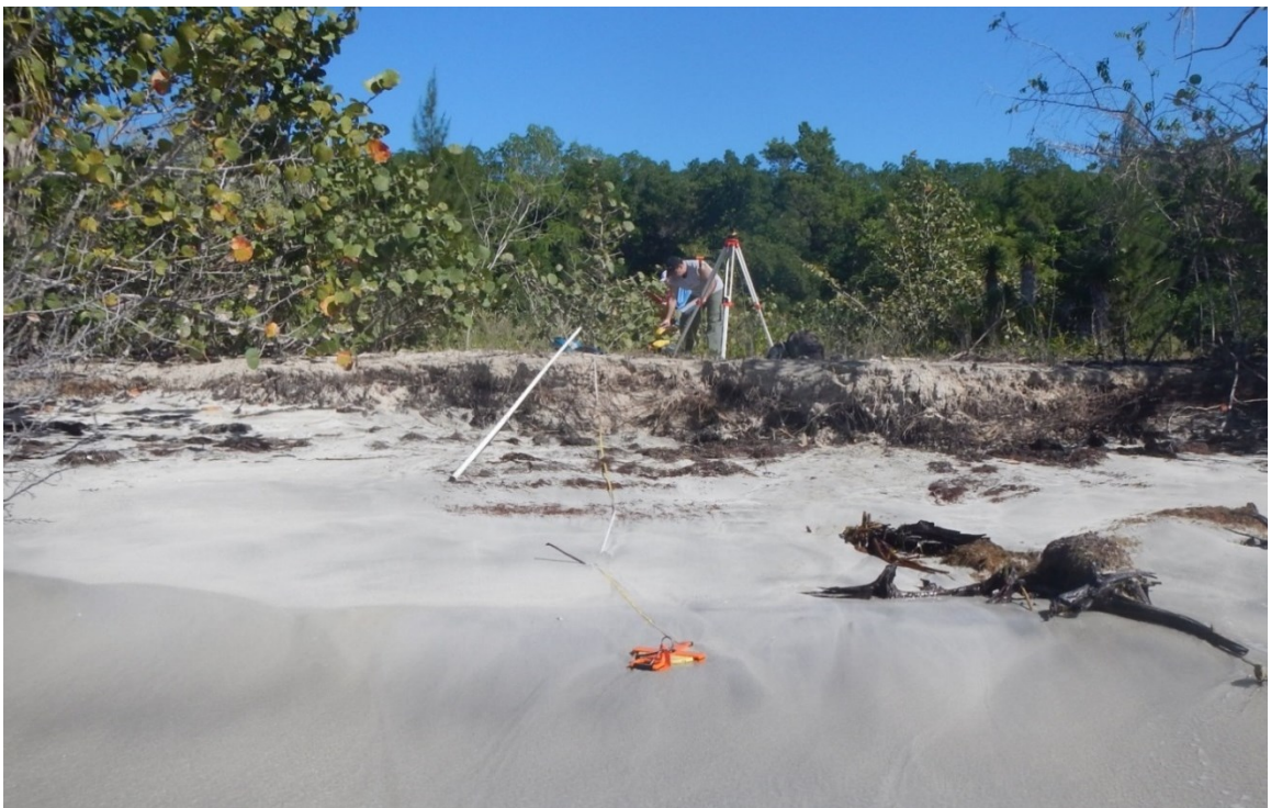
Site 16, Transect 1: An example of an eroding beach with an active scarp.
