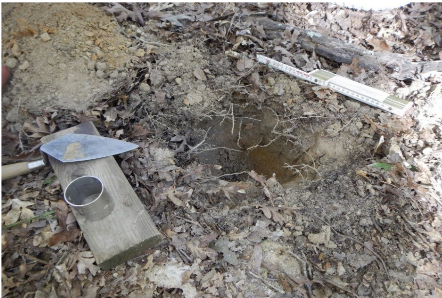
Appendix C-8. Site 1 subplot 2, oak unburned stand; bulk density ring and sampling tools; October 2015.
