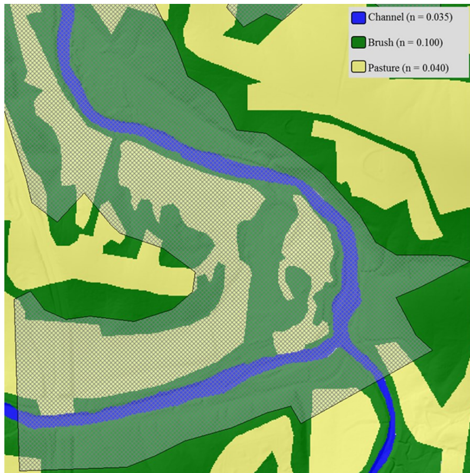
Figure 18 - Land use layer and defined Manning's n layer used for HEC-RAS modeling.
