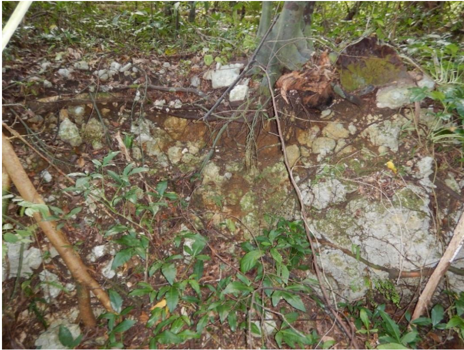
Appendix B-12. Point 9 – Bedrock Wall on Left Bank of Incised Channel, Fine Sediment Within the Channel Was Eroded in 1979
