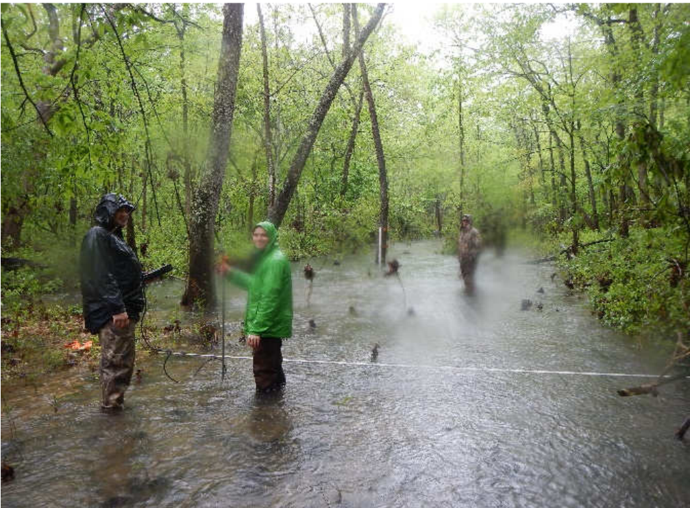
Figure 8D. Collecting discharge measurement with SonTek FlowTracker at the MBBC gage location (site-4).
