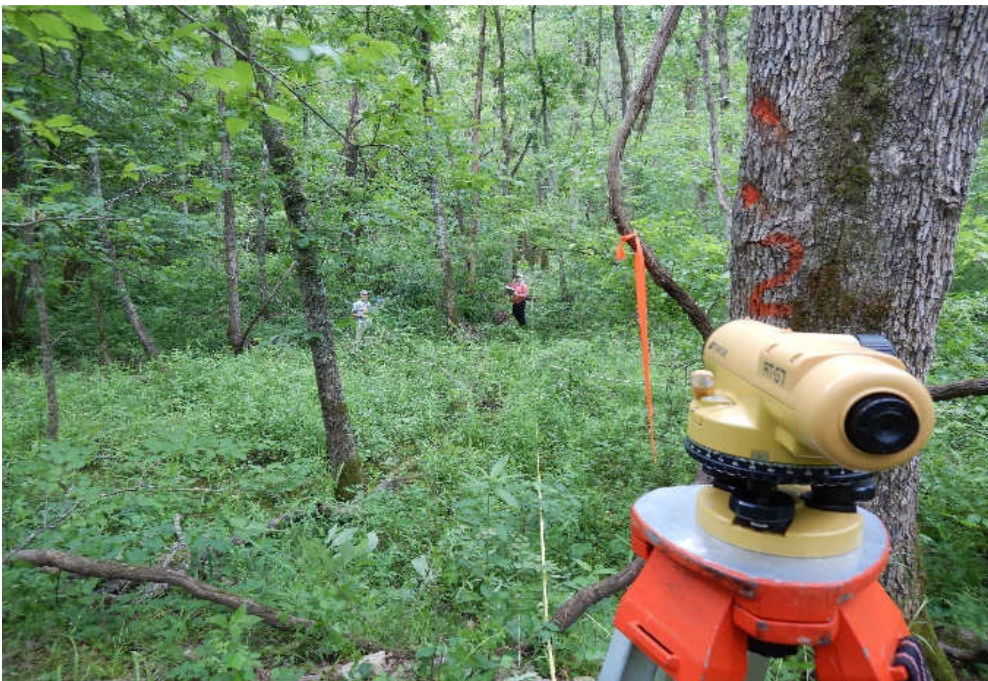
Figure 8B. Channel cross-section survey at site-2 using an auto-level.
