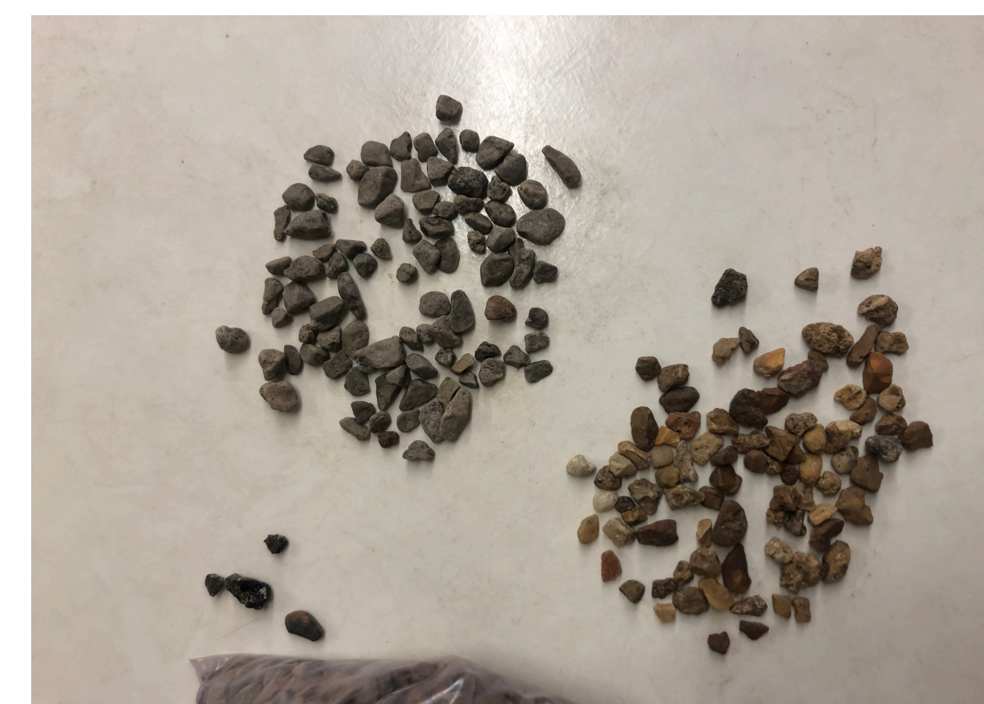
Figure 7: (Above) Shows a sub-sample from a 4-8 mm size fraction that has been separated based on dolomite fragments (left) and all other sediment grains (right)
