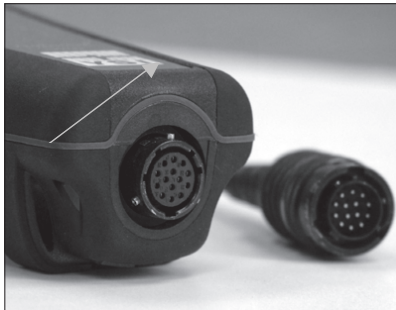
Figure 5. Note the keyed connector. The cable and instrument connectors can only be mated once the keys are properly aligned.
