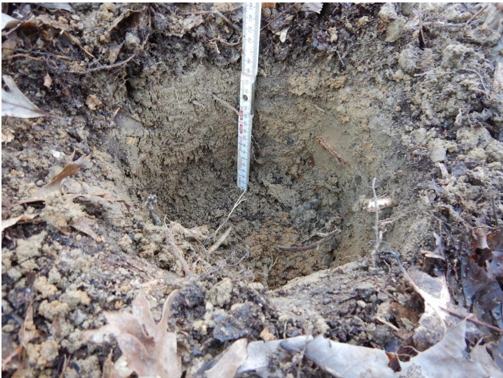
Photo 24. Example of a soil sampling point with the “O” horizon present (Wild Coyote: December 6, 2019).
