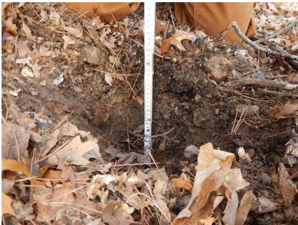
Photo 12. Rocky colluvium material above loamy A horizon (Warthog: April 5, 2018).
