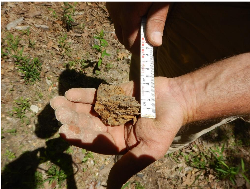
Photo 7. Using an example of platy structure to help field workers identify it in the field (Monterey: May 11, 2018).
