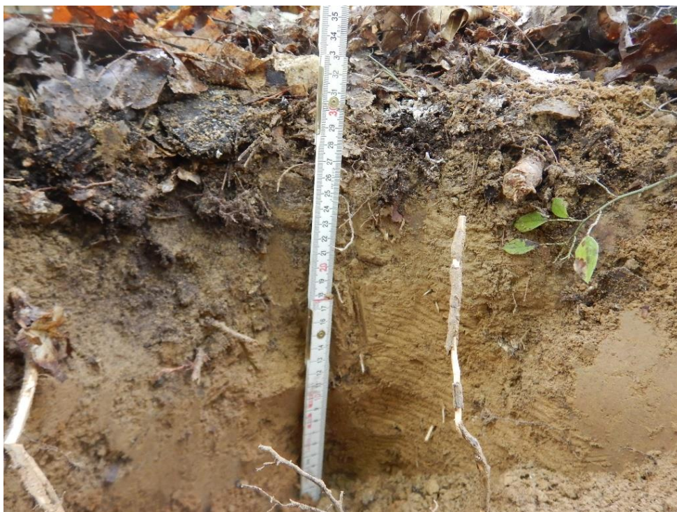
Photo 14. Loess parent material (Wild Coyote: Sept. 27, 2018) NOTE: Horizontal lines are not platy structure but are from scraping with a soil knife.
