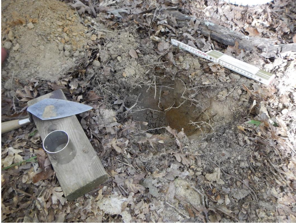
Photo 5. Preparing an area to take a soil bulk density sample with the bulk density ring.
