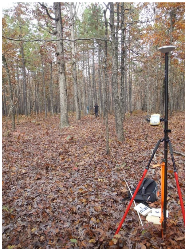
Photo 2. Center stake and transect being used to establish other subplots, device in center is the RTK used to obtain GPS data.
