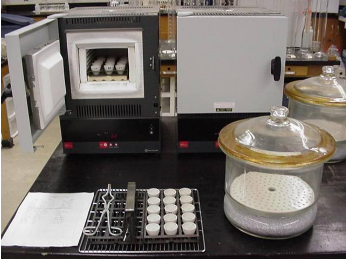
Figure 11. Muffle furnaces in the SMSU Geomorphology lab.
