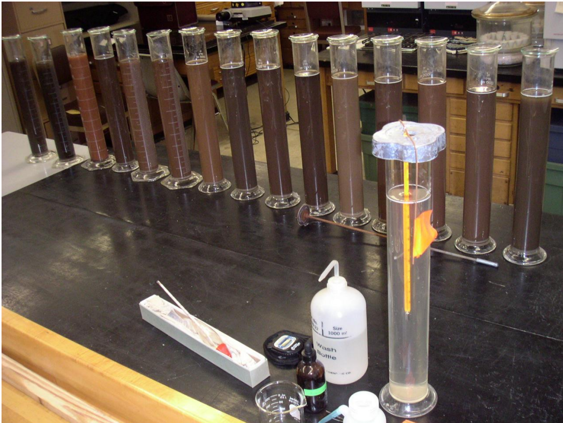
Figure 12. Sediment suspended in one liter cylinders for hydrometer readings.
