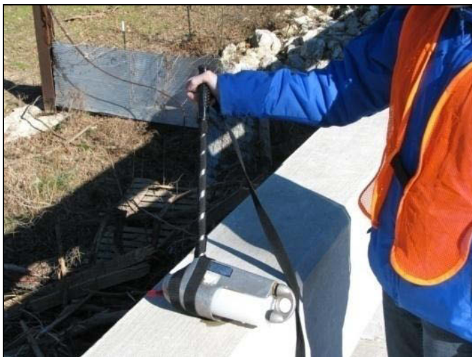
Figure 4.1. US DH-48 depth-integrated sampler
