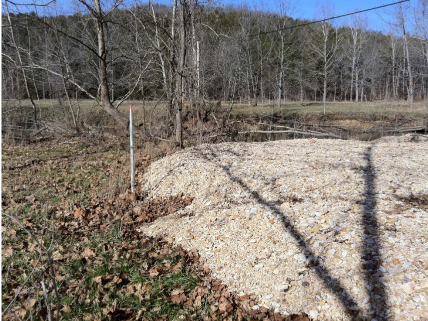
Gravel splay over bankfull height. 2meter stadia rod in photo at flood plain height.
