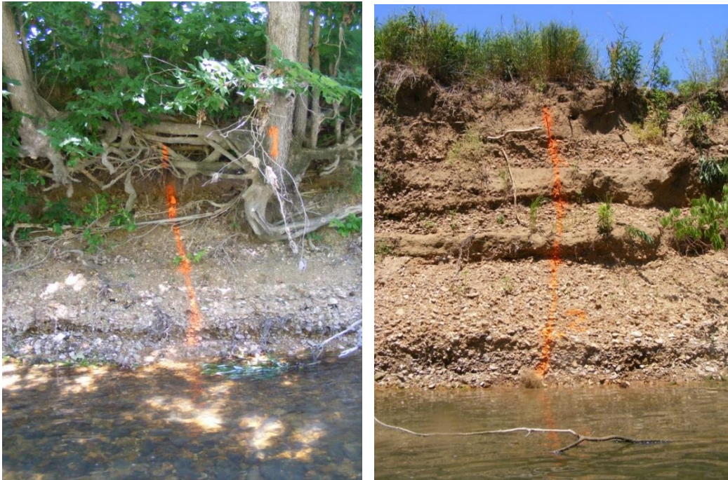
Figure 36. Pin arrays one and two. This area of the bank was composed of previously deposited gravel that can lead to higher erosion rates (August, 2012).
