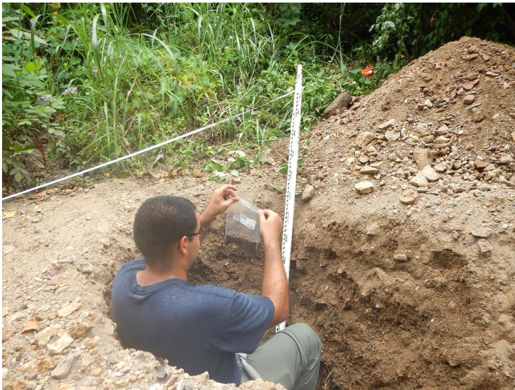
Stable bar core sampling at R-km 4.25.
