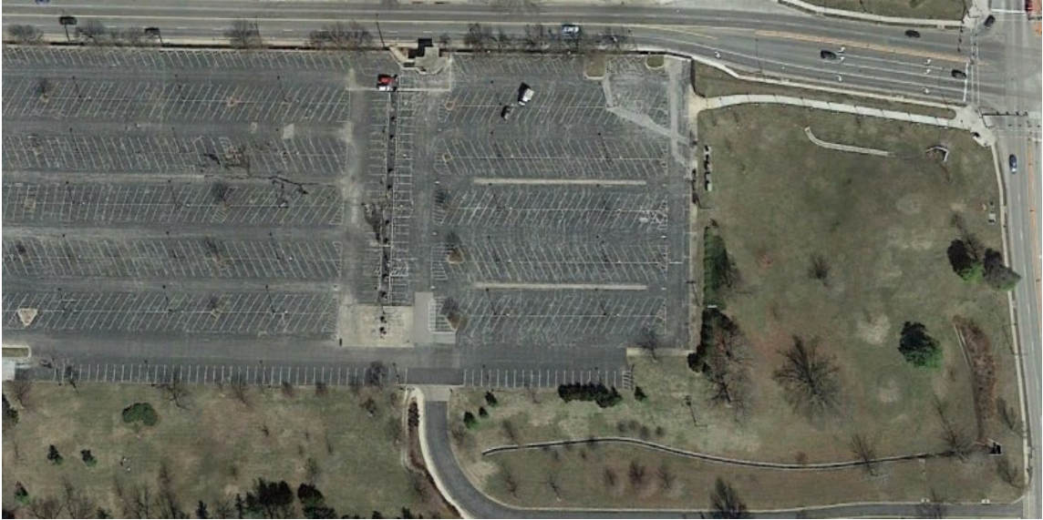
Fig. 1. Parking lot (2011) with coal-tar sealant (A) and (2015) abraded coal-tar sealant (B). Sealant particles formed by weathering and vehicle abrasion are released to local waterways during storm events.
