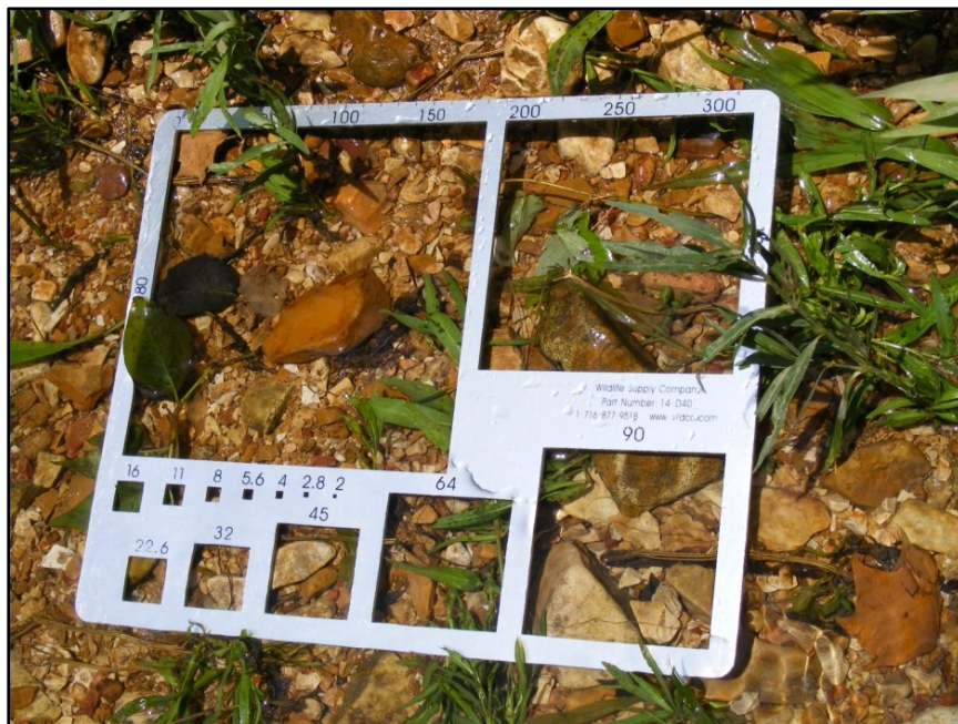
Figure 12. Gravelometer used in pebble counts.
