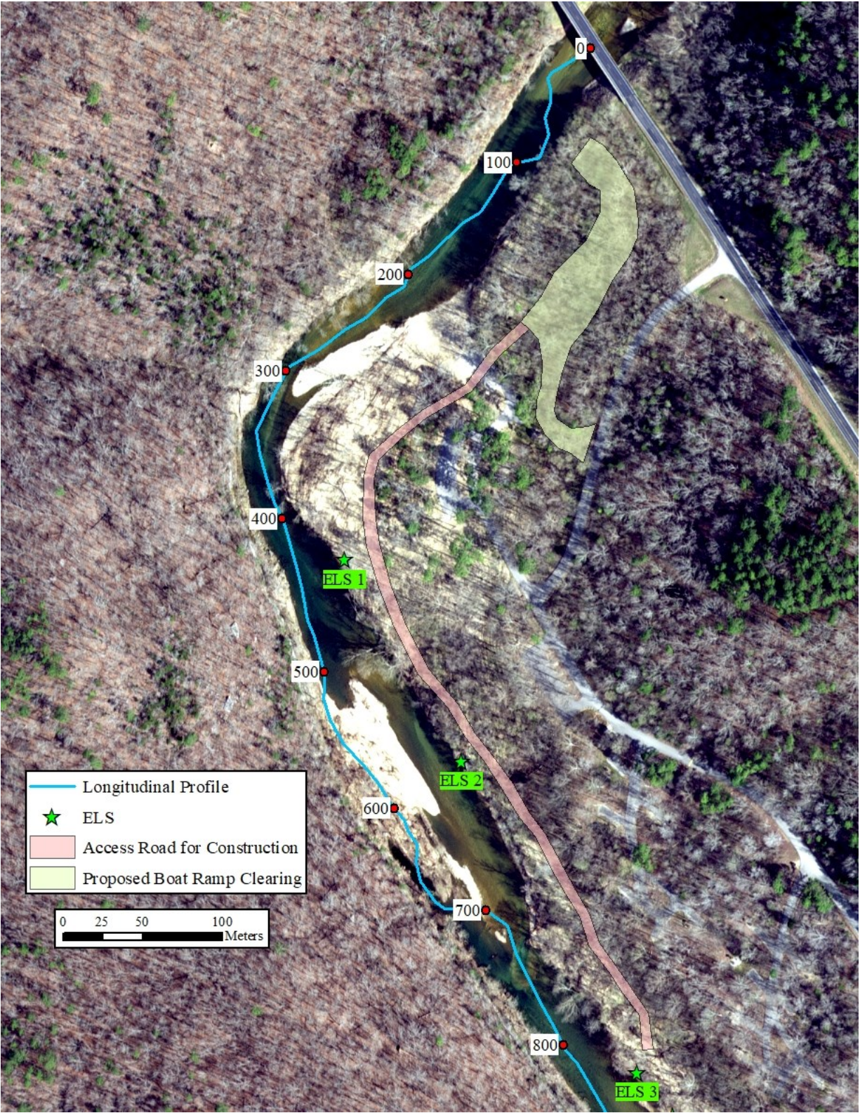
Figure 20. Construction disturbance to the North Fork Recreation Area including clearing for proposed boat ramp and construction access road (MDNR, 2015).
