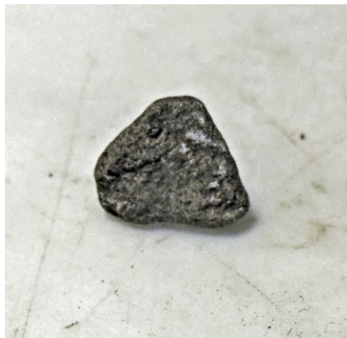
Figure 11: Typical Old Lead Belt coarse tailing. Milling processes produced distinctively blue-grey, angular waste sediments.
