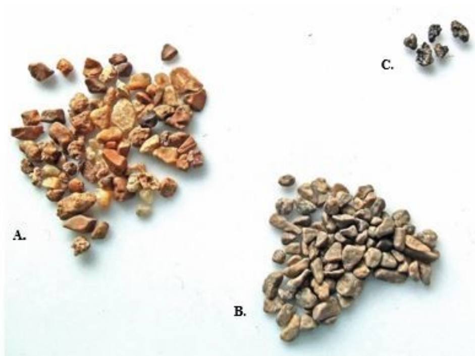
Figure 12: Lithologic classification of grains in Big River channel sediments (4-8 mm). From left to right: A) natural sediment composed of chert and other silicate minerals, B) chat grains Bonne Terre dolomite from processed, and C) coal/slag pieces.
