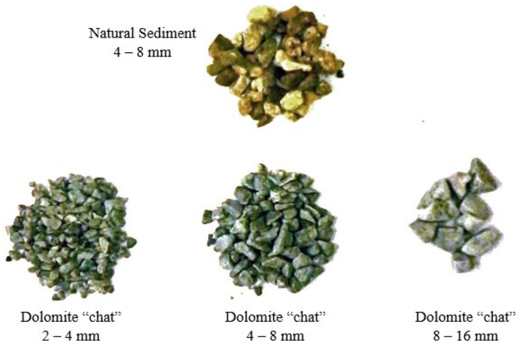
Figure 18: Dolomite chat size fractions in Big River bar deposits. Natural (chert/quartz) sediments are shown in contrast to the dolomite waste sediments.
