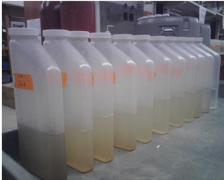
Figure 5. Samples collected from the PS show the change in suspended solids throughout the storm event.
