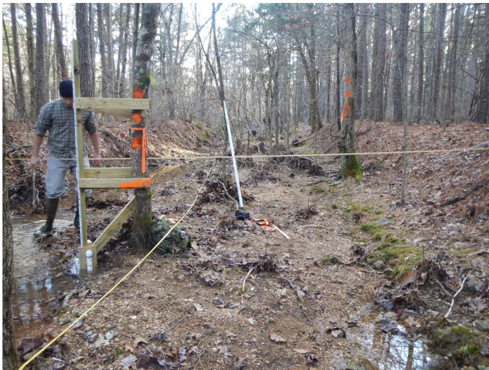
Photo 2. Water level stage recorder and staff gage installed at Barnes Hollow (12/14/2015).
