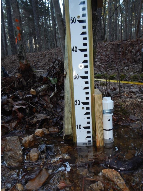
Photo 3. Water level stage recorder attached to stage gage at Barnes Hollow (12/14/2015).
