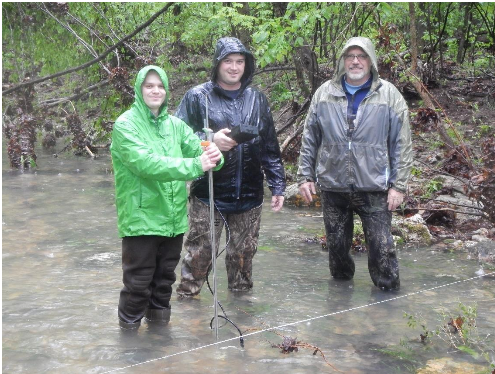
Photo 6. Collecting discharge measurements with SonTek FlowTracker at the Fools Catch gaging station for calibrating rating curves (05/05/2017).
