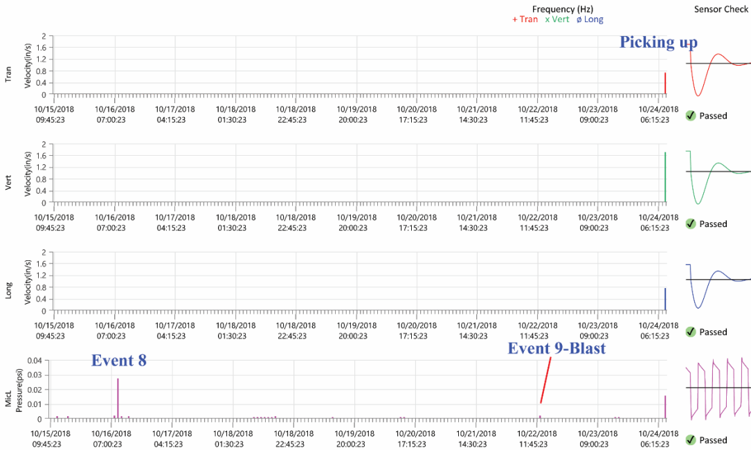
Figure 7. Output from the InstanTel Blastmate seismic and sound recorder: October 15 to 24, 2018. The bottom graphs show seismic events on the vertical (vert), transverse (Tran) and longitudinal (Long) components in in/s, and the sound events from the linear microphone (MicL) in psi. Three significant events are marked on the graphs.
