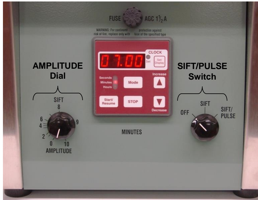
Photo 2. Sonic Sifter control panel.
