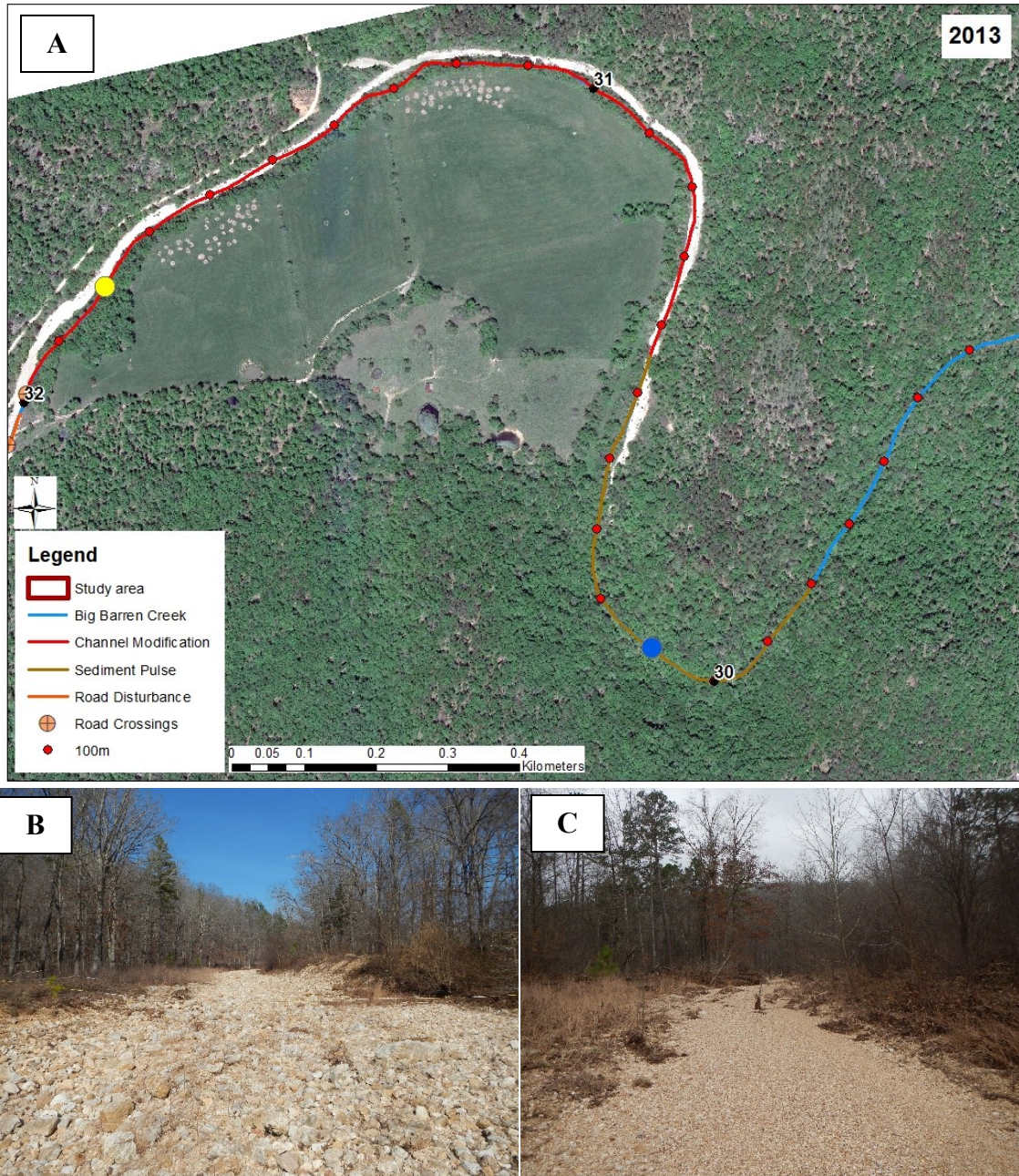
Figure 16 - Map of channelization from 37.7 to 37.1 km. A: Aerial photo (2013) of channelized segment 34.0 to 30.55 km and subsequent sediment pulse to 29.8 km. B: Ground-truthing photo (2016) of channelization 31.8 km denoted as yellow circle in A. C: Ground-truthing photo (2016) of sediment pulse at 30.1 km denoted by blue circle in A.
