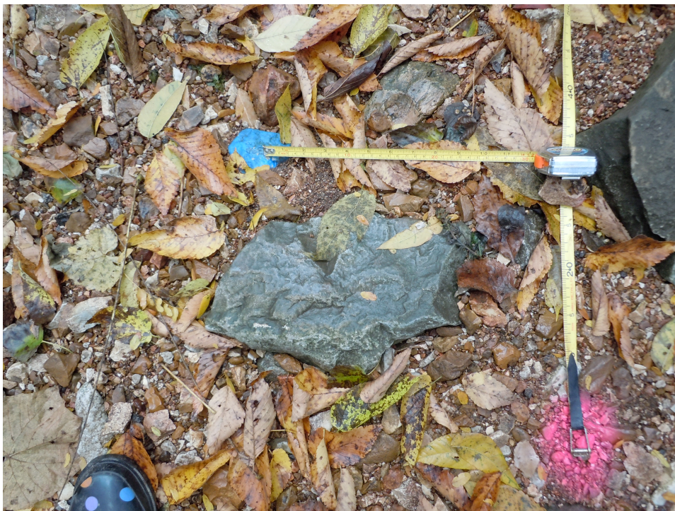
Figure 3.9 Taking a measurement from deployment site to tracer position after flow event.
