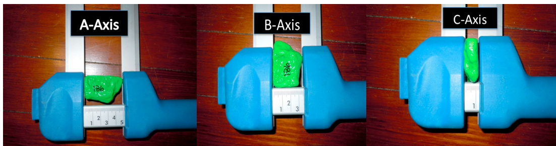
Figure 3.7 Axis dimensions for pebble size measurements (cm).
