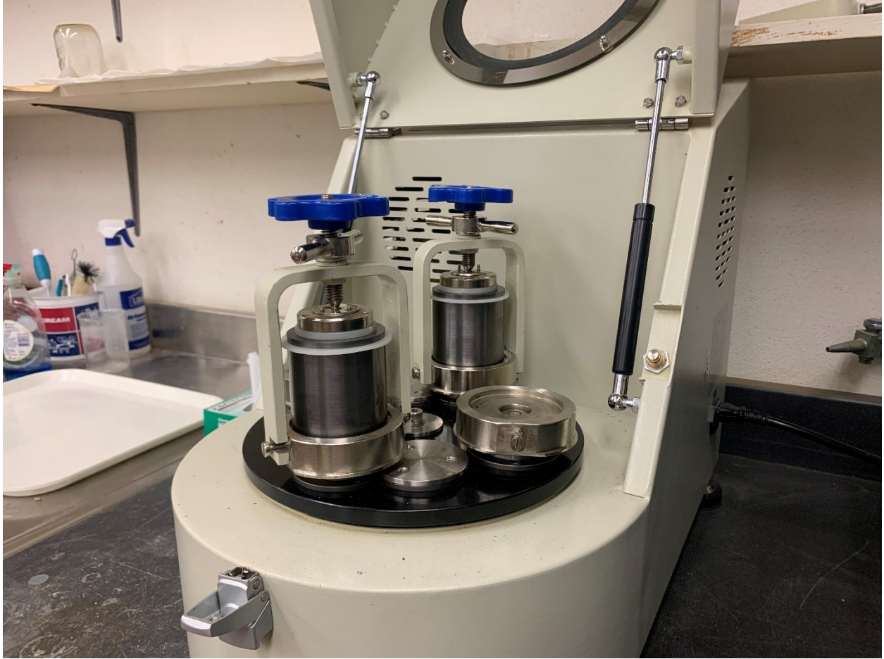
Figure 11. The ball mill used to crush coarse sediment into a fine powder.
