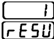
2. If running a program from a Model 750, use the UP or DOWN arrow keys to cycle the Actual display to the desired program *number*, 1 through 4, or NO to cancel. Use the MENU key to select the desired program *number* to run.
