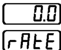
10. The Set Display then indicates "rAtE" to prompt the operator to select a desired heating or cooling rate in °C/min or °F/min. Press and hold the UP or DOWN Arrow key until the desired rate is shown in the Actual Display.
