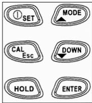
1. **⓪ (POWER) SET button:** Press to power on meter. When meter is on, press and hold to enter setting {SET} mode. Press this button again to turn off.
