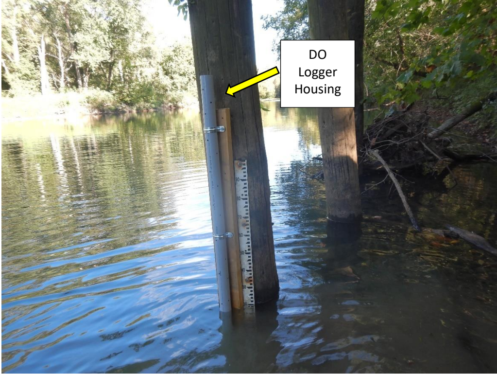
Photo 3. DO sensor housing at BPD (9/23/2019).
