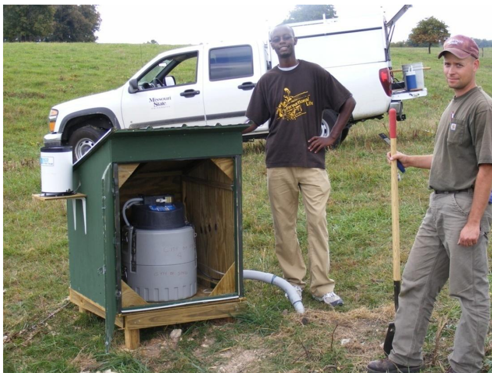
Photo 11. Auto-sampler and Rain Gage Installation (October 2008)
