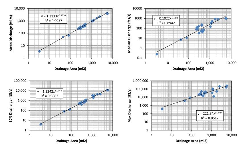
Figure 14. Drainage area and discharge relationships for 25 USGS gaging stations near the study watershed.
