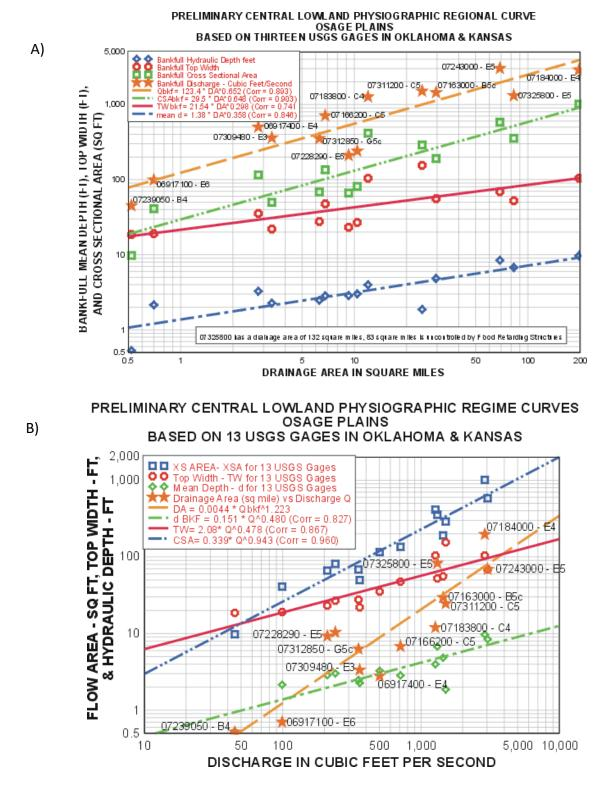
Figure 6. Preliminary A) regional and B) regime curves for the Osage Plain physiographic region. Source: NRCS-National Water Management Center <u>www.nrcs.usda.gov/wps/portal/nrcs/detail/national/water/manage/hydrology/?cid=nrcs14</u> <u>3 015052</u>
