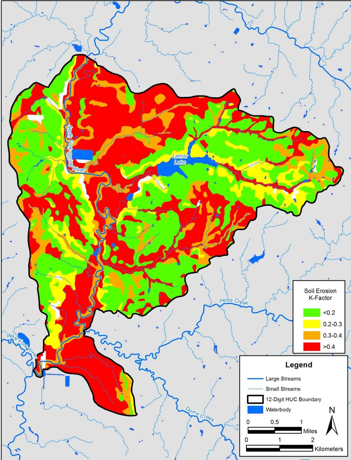
Figure 12. Soil series classified by soil erosion K-factor.
