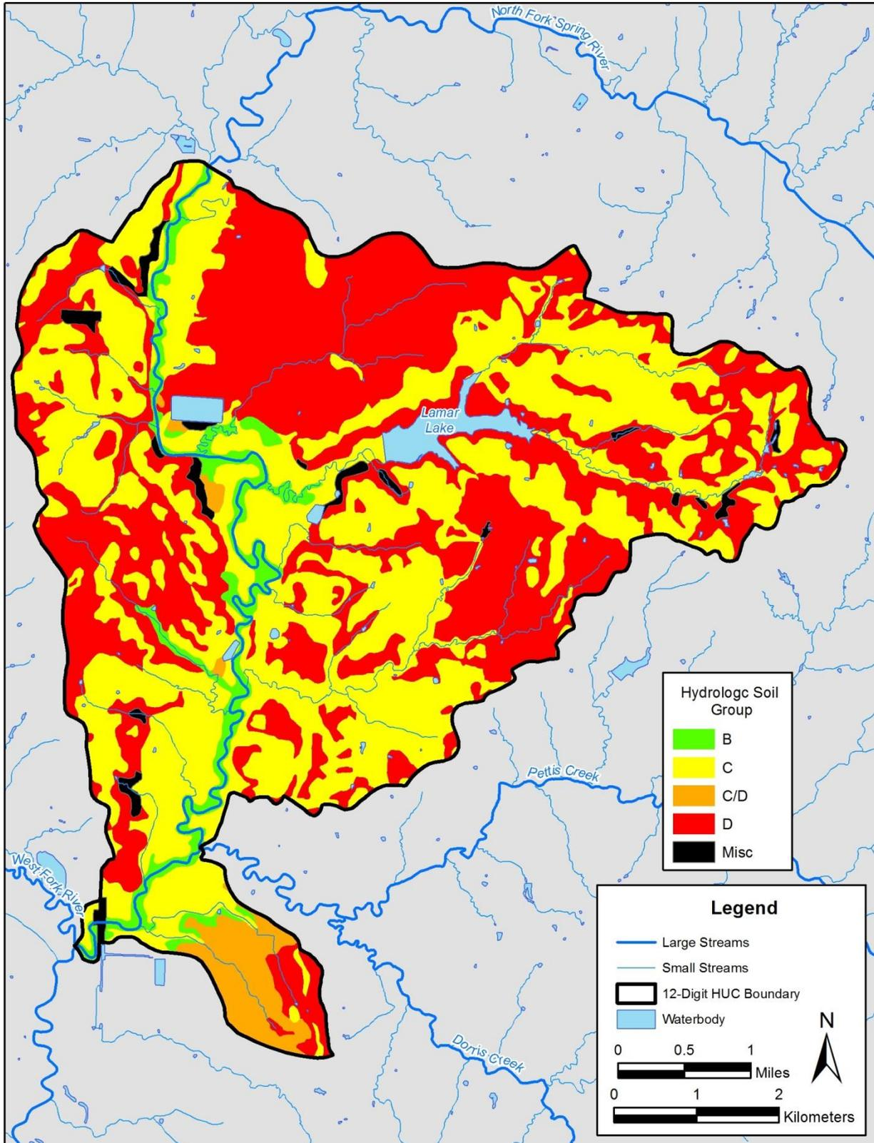
Figure 10. Soil series classified by hydrologic soil group.
