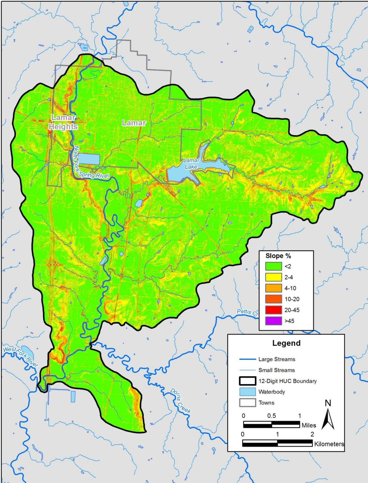
Figure 8. LiDAR based slope classification across the watershed.
