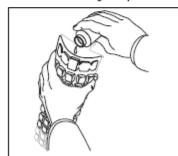
Pour the reagent/sample mixture directly into the Quanti-Tray avoiding contact with the foil tab. Tap the small wells 2-3 times to release any air bubbles. Allow foam to settle.
