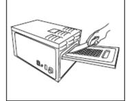
Place the sample-filled Quanti-Tray onto the Quanti-Tray/ 2000 rubber insert of the Quanti-Tray Sealer with the well side (plastic) of the Quanti-Tray facing down.
