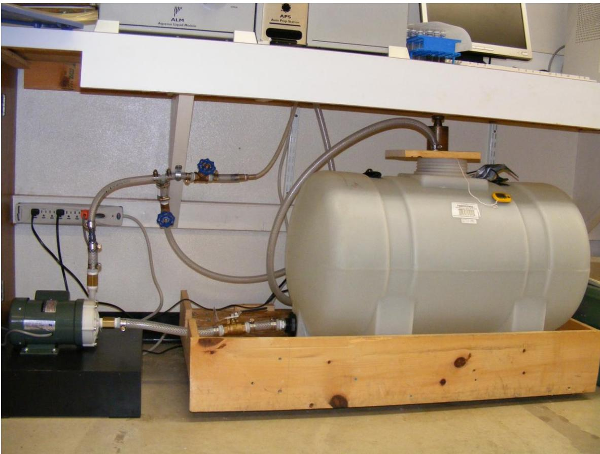
Photo 1. Water Tank Assembly for Beckman Coulter LS 13 320.
