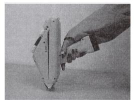
Figure 6. Correct Procedure: Use of the appropriate 90° angle of measurement.
