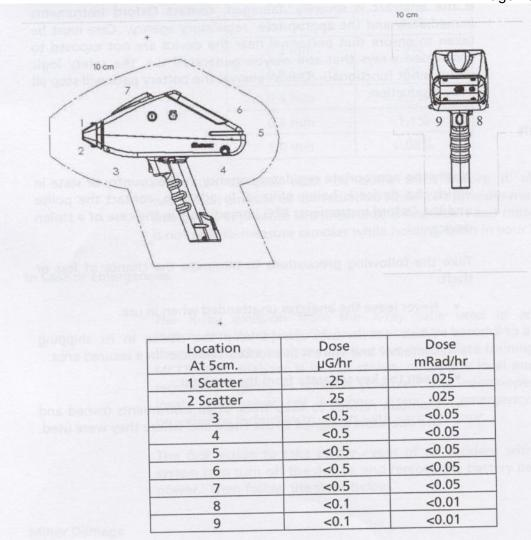
Figure 2. Background Radiation Measurements: These measurements indicate that the air kerma rate at 5cm form any accessible surface was lower than 4.38 µGy/hr.
