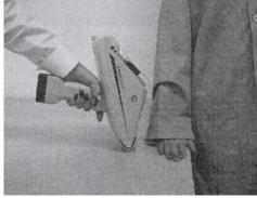
Figure 1. Incorrect Procedure: All persons not directly involved in operating the instrument will remain three feet away from the instrument during analyses.
