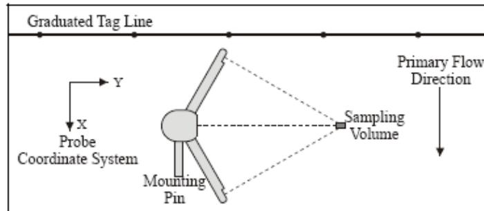
Figure 2: Velocimeter placement perpendicular to the tape line.
